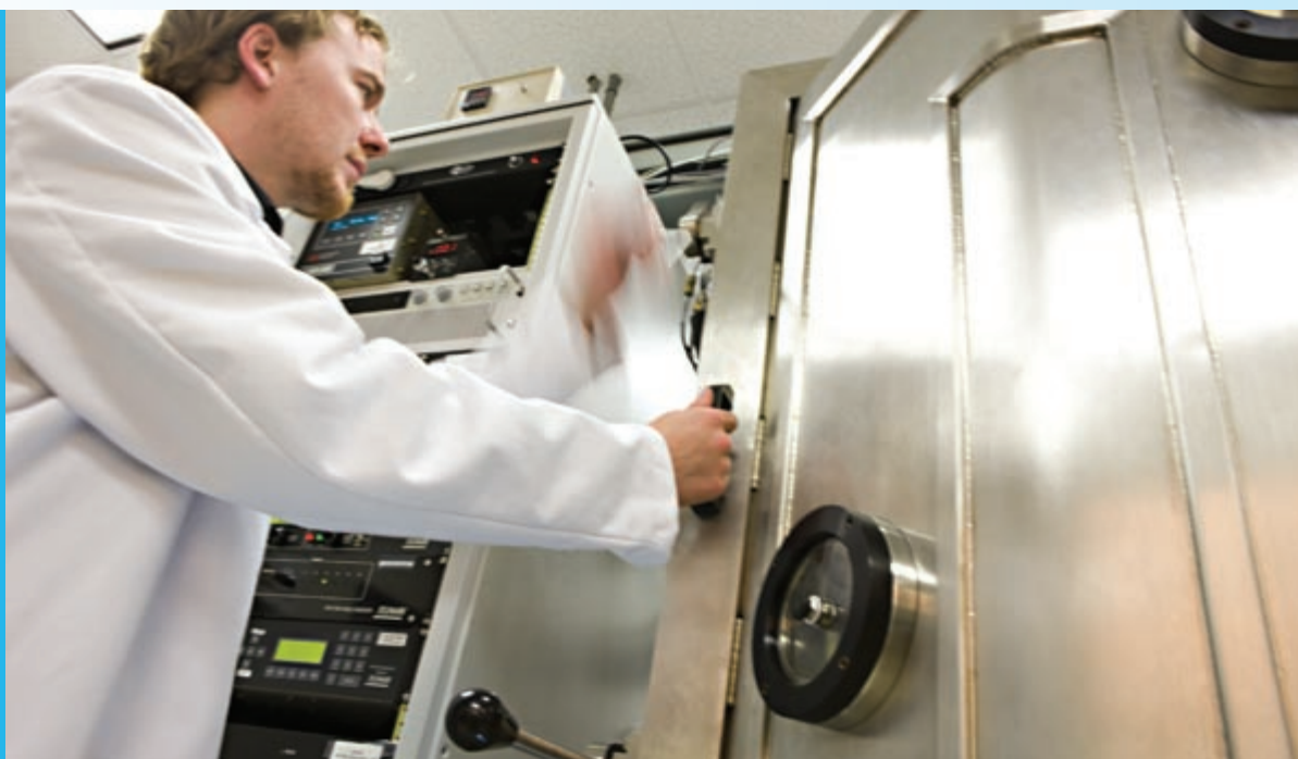
THOMAS GUSTAFSON, INTERN, PREPARES THE ION BEAMS ASSISTED DEPOSITION (IBAD) SYSTEM THAT PRODUCES THE NANOCRYSTALLINE COATING.
