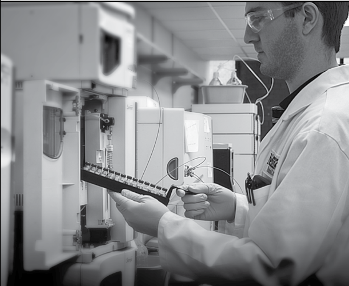
JOHN WEINHOLD, RESEARCH TECHNOLOGIST, ANALYZES DRUG CONCENTRATIONS IN BLOOD SAMPLES USING A MASS SPECTROMETER IN DR. FLETCHER'S LAB.
