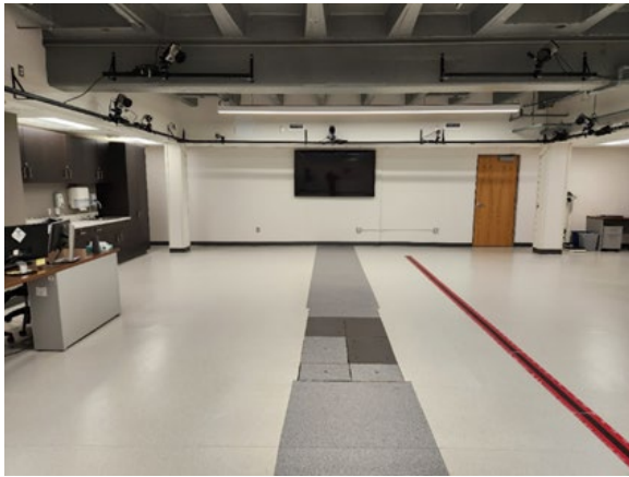
Force plates embedded in the floor with motion analysis cameras mounted around the ceiling.
