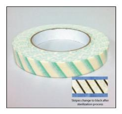
Lead free or Lead/Latex autoclave tape is available for purchase through UNMC's eShop (Fisher Scientific catalog # 10153-152 respectively). This tape clearly indicates that it is lead free. It has green lines that turn dark after 15 minutes of exposure to a temperature of 121°C (250°F) in a steam autoclave.
