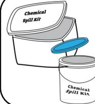
Bin, bucket, or bag to store kit items. The container must be clearly labeled as a Chemical Spill Kit.
