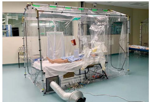
ISTARI, a low-cost, mobile, modular structure that drastically reduces PPE needs.
