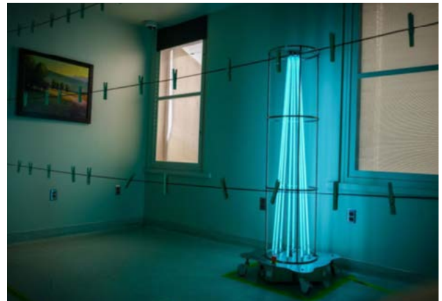
UV light decontamination process developed to reuse N95 masks
