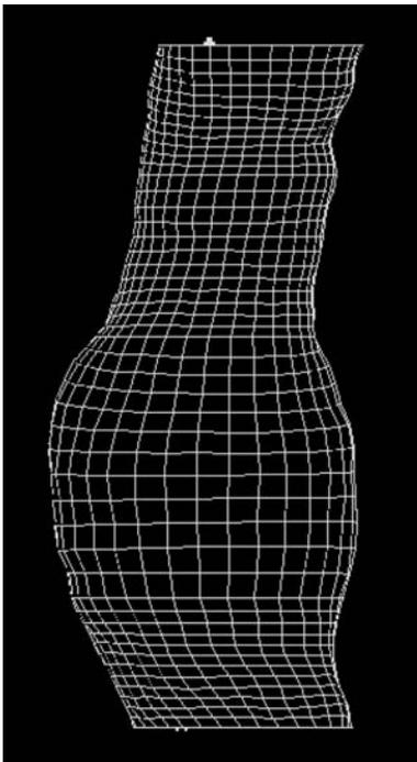
**Figure 2.** Computational grid of the AAA model used for the finite-element analysis.
