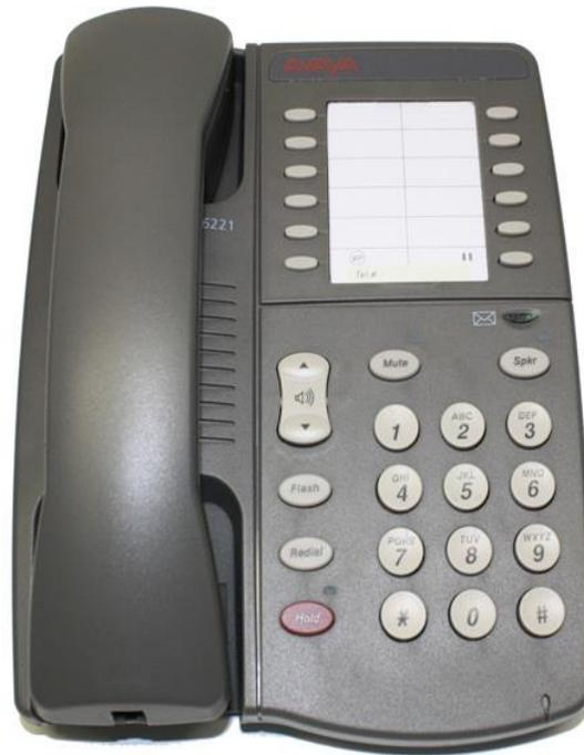
The **6221** is a one line Analog phone with ten programmable dialing buttons, and has an integrated speakerphone. The phone can also be wall mountable
