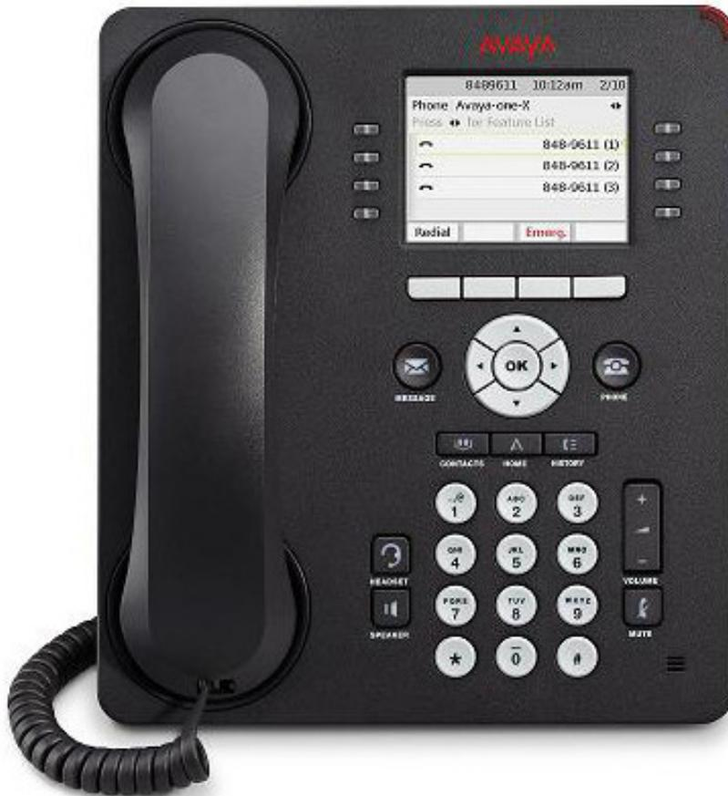
The **9608/9608G/9611G IP** supports 24 programmable call appearance/feature buttons, has 8 physical buttons, 4 softkeys, USB port, and a two-way speakerphone. The phone is also wall mountable.
